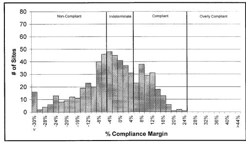
Figure 6: Compliance Results - AB 970 Standards - HERS-Certified Duct Sealing
