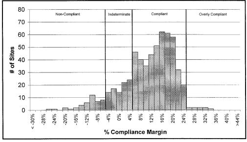
Figure 5: Compliance Results – AB 970 Standards – Low Solar Heat Gain Fenestration (0.35) and High Efficiency Air Conditioning and High Efficiency Water Heating
