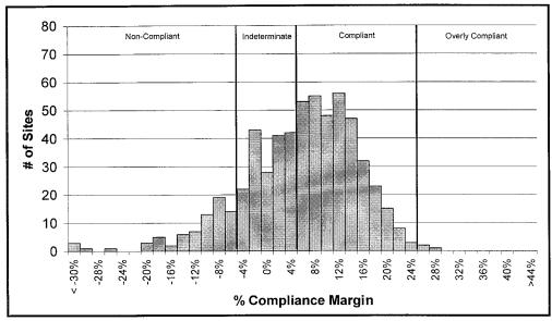
Figure 7: Compliance Results – AB 970 Standards – HERS-Certified Duct Sealing and TXV Valves and High Efficiency Air Conditioning and High Efficiency Water Heating
