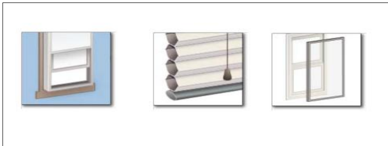
Figure 1. Examples of Window Attachments - Exterior Storm Window, Cellular Shade, and Interior Window Panel (Lawrence Berkeley National Laboratory)
