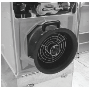
Figure 2: Fan Assisted Flow Meter “Reference” (Not used in study)
