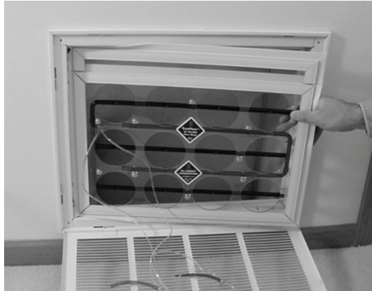
Figure 1: Orifice Plate Air Handler Flow Meter “Flow Grid”
