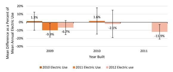
**Figure 9.** Mean differences in modeled vs. normalized annual electric use over time as a percent of mean annual usage, in electric heated EPS homes built from 2009-2011. Note: positive values indicate that models overestimated usage, on average, while negative values indicate that they underestimated it.
