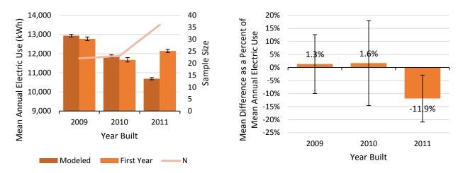
**Figure 7.** Comparison of mean modeled vs. first year normalized electric use (in kWh) and mean differences as a percent of mean annual usage in electric heated EPS homes built from 2009-2011. Note: positive values indicate that models overestimated usage, on average, while negative values indicate that they underestimated it.
