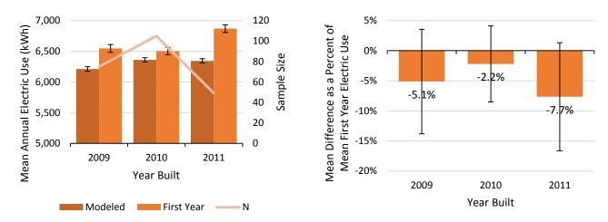
**Figure 3.** Comparison of mean modeled vs. first year normalized electric use (in kWh) and mean differences as a percent of mean annual usage in gas heated EPS homes built from 2009-2011. Note: positive values in the graph of differences indicate that models overestimated usage, on average, while negative values indicate that they underestimated it.
