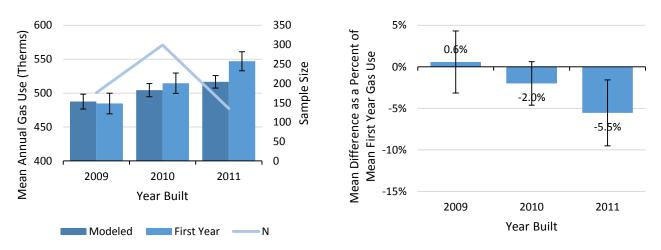
**Figure 1.** Comparison of mean modeled vs. first year normalized gas use (in therms) and mean differences as a percent of mean annual usage in gas heated EPS homes built from 2009-2011. Note: positive values in the graph of differences indicate that models overestimated usage, on average, while negative values indicate that they underestimated it.
