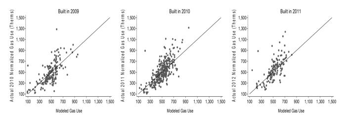
**Figure 2.** Scatterplots of modeled gas usage versus the deviation in first year normalized gas use from modeled usage (in therms) for individual gas heated EPS homes built from 2009-2011. Note: the reference line indicates where first year and modeled gas use are equivalent; points above the line indicate homes where actual usage was higher than estimated and vice versa.
