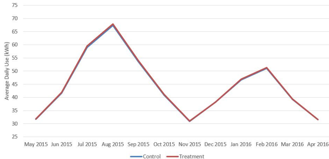
Pre-Intervention Average Daily Energy Use (kWh) Matching on Energy Use & Age
