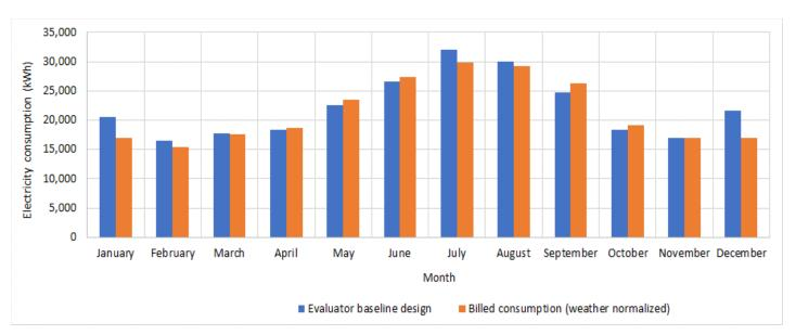
Example of a site-specific baseline model calibrated to facility consumption
